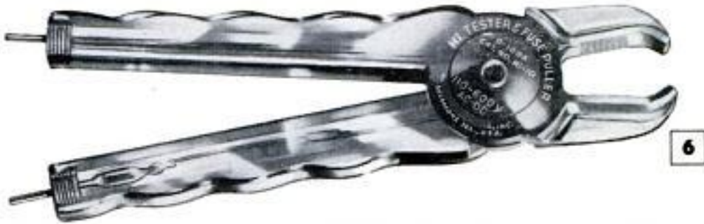
6. FUSE PULLER combines a circuit tester for use on 100 to 600-V. lines a.c. or d.c. Electrodes are in the handles. One glows on d.c. and both glow on a.c. Both are replaceable. Handles fuses up to 100 amp.
